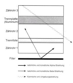
A high energy Alpha-particle will trigger an event in the two lower detectors ZR1 and ZR2 depicted here on the left. Because both events occur quasi simultaneously these events can be eliminated with an Anti-coincidence gate. This will eliminate the majority of natural Alpha's from the first detector ZR1 and only leave the artificial Alpha's. An artificial Alpha-particle is prevented from entering the second detector ZR2 by absorption in the separating foil between the 2 detectors.
