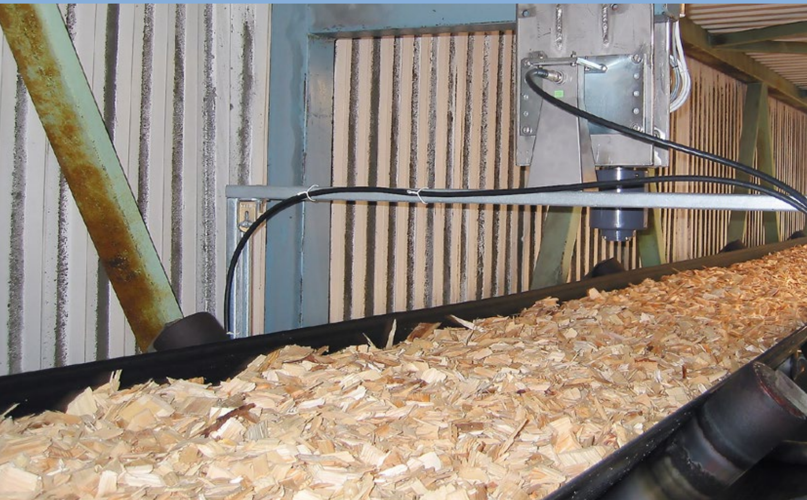
Moisture measurement of wood chips – LB 568 with horn antennas and radiometric area weight compensation.
